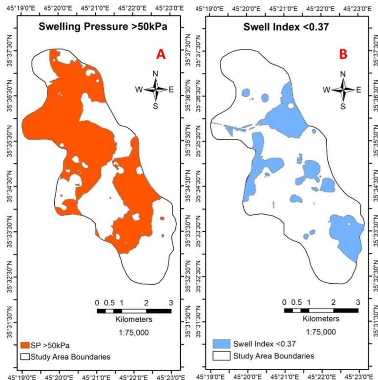
**Figure 11.** Zones of high swelling potential soil at the study area for A (SP>50 kPa) and B (SI<0.37)
