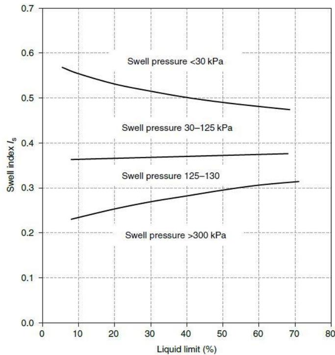
Figure 3. Relationship between liquid limit and swell index for expansive soil (Murthy, 2002; Chen, 1988)
