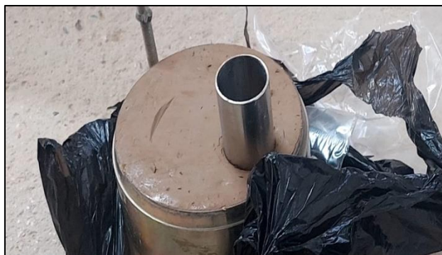
Figure 3. Mechanism of unconfined sample extraction
