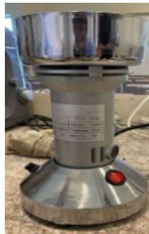
Figure 10. Grinding equipment used to pulverise pumice aggregate.
