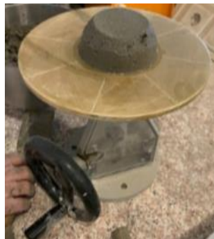
Figure 8. Flow table test for cement mortar of control sample.
