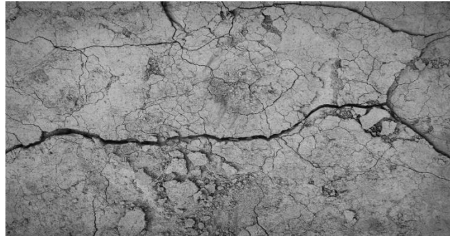
Figure 4. Shrinkage of cement mortar (Patel, 2017).
