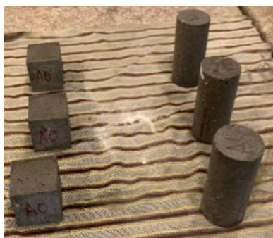
Figure 12. Cement mortar cubes before compression testing.
