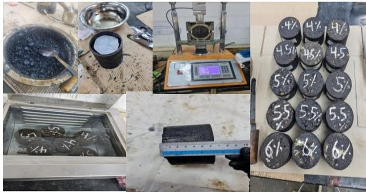
**Figure 4.** Marshall specimens prepared and tested sequences.
