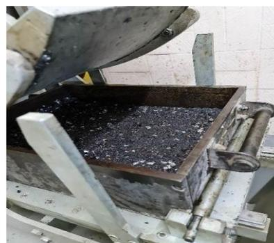
**(c).** Casting the loose mixture.
