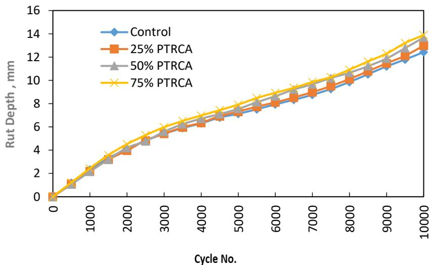
Figure 9. Rutting depth(mm) at 10000 cycles.
