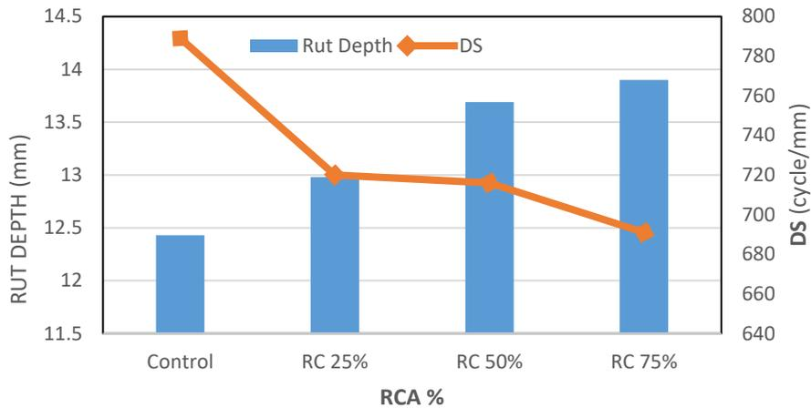
Figure 10. Relation between dynamic stability and rut depth and RCA.
