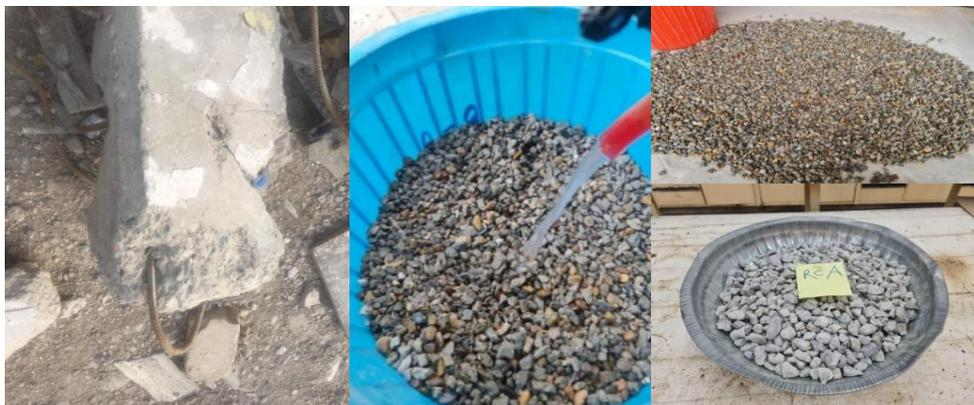
**Figure 2.** Concrete waste and RCA particles.
