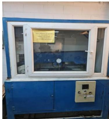
**Figure 5.** Wheel-tracking device at the University of Baghdad.
