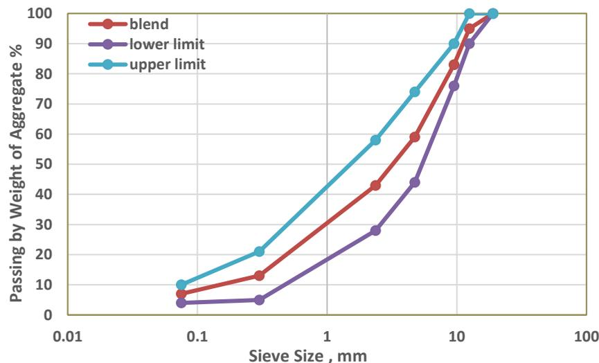
**Figure 1.** Aggregate gradation by (SCRB R/9, 2003).
