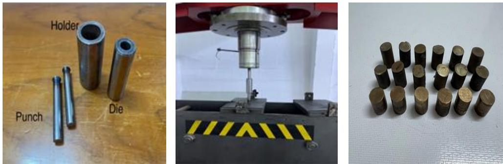
**Figure 3.** Tools used to manufacture the samples, the compression machine, and the samples after compression.
