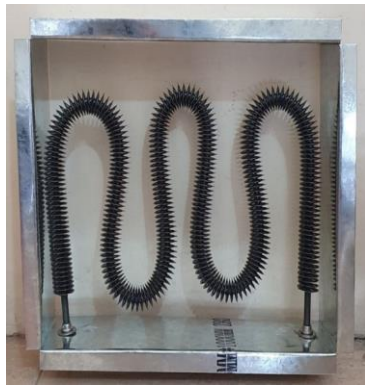
Figure 2. finned heater with a capacity of (2500W)
