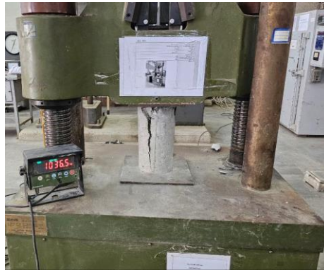
Figure 5. ECC compressive strength test
