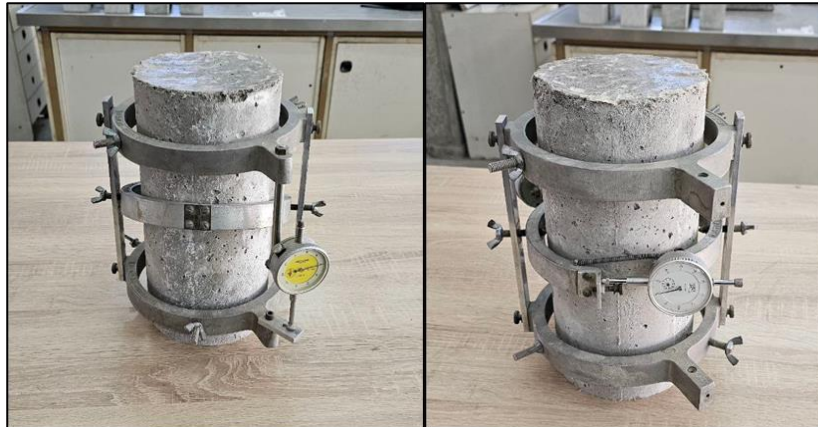
Figure 9. Static modulus of elasticity test of ECC samples
