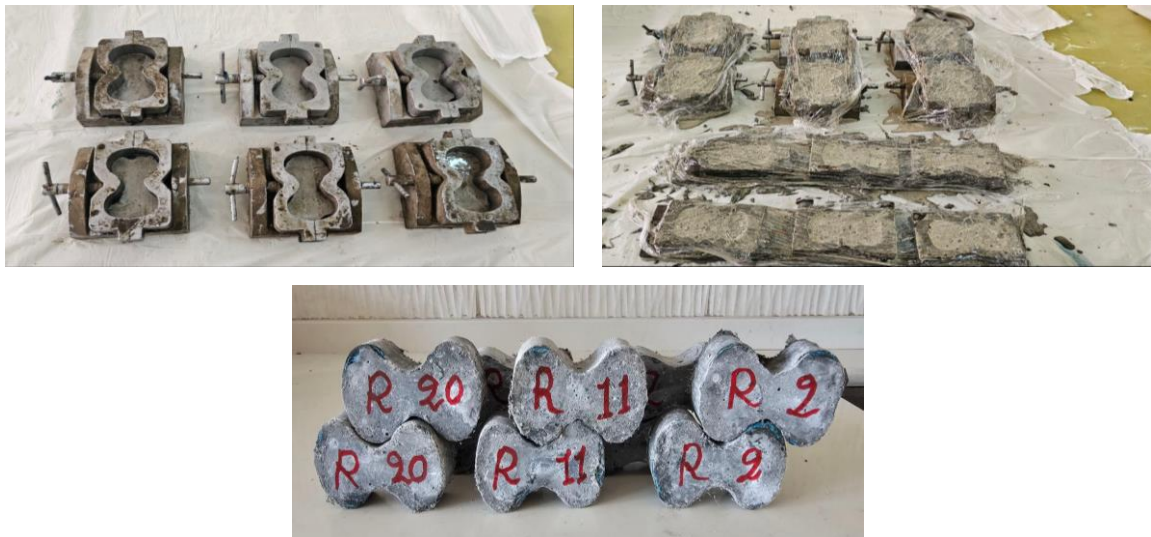
Figure 3. Dog-bone specimens of SCC-ECC mixtures (R2, R20, and R11) prepared for direct tensile strain-hardening test.
