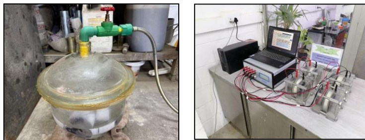
Figure 12. Chloride penetration test of SCC-ECC sample
