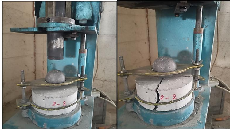
Figure 7. ECC specimen under impact load – before and after failure
