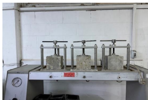
Figure 8. Water Permeability Test of ECC Samples
