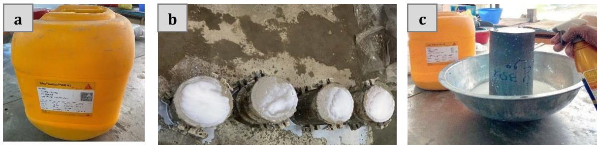
Figure 9. Liquid-membrane compound (LMC): (a) Sika Antisol-WB, (b) Sprayed on the top of the surface, (c) After being taken out of the mold
