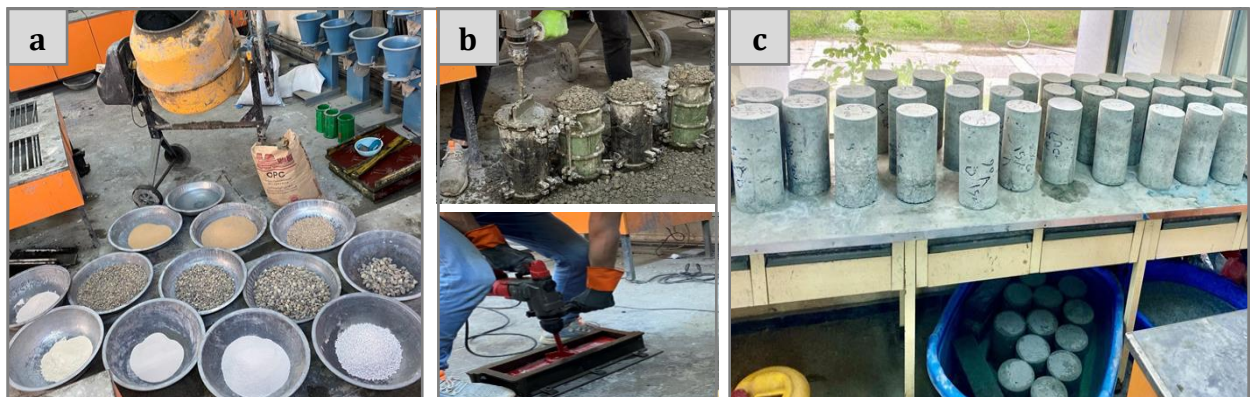
Figure 5. (a) Preparing material and mixing, (b) The compaction for cylinder and prism, (c) The samples after casting
