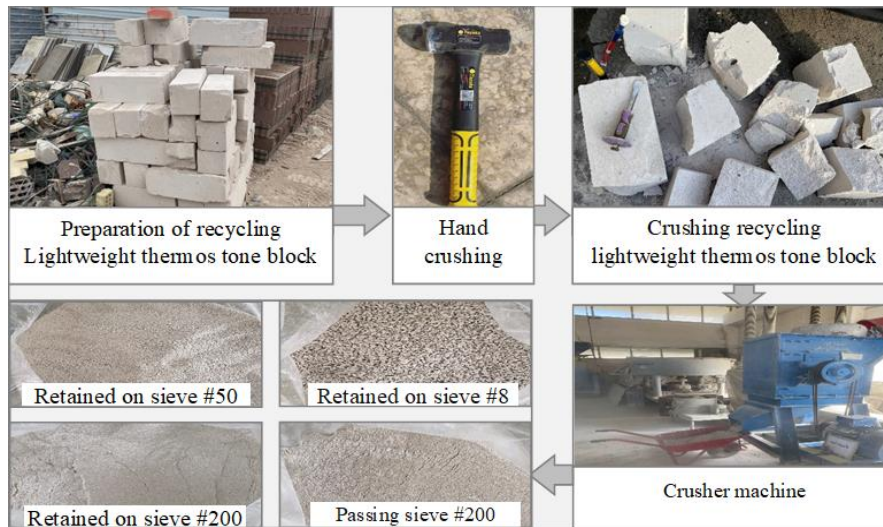
Figure 3. The steps of preparation waste thermostone block (WT)
