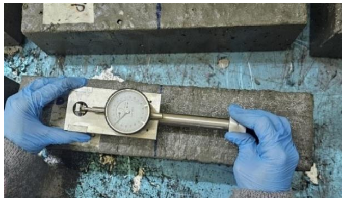
Figure 5. Drying Shrinkage Test by using an Extensometer
