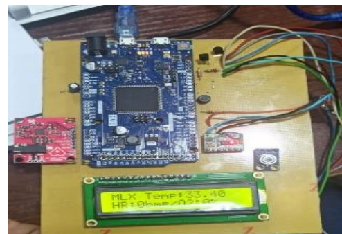
Figure 4. Depicts the final design of the printed circuit board after attaching the sensor devices to the Arduino.
