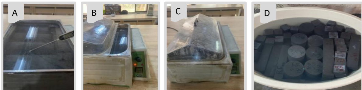
Figure 3. Thermal curing process: (A) initial heating stage, (B) raising the temperature to 70°C, (C) maintaining the specimens at 70°C for 5 h, and (D) normal water curing
