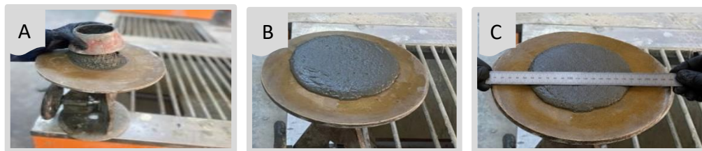
Figure 2. Flow table test: (A) before flow, (B) after flow, and (C) diameter measurement.
