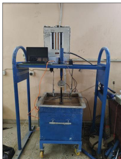
Figure 5. Laboratory arrangement used for static loading of untreated and improved clay models.
