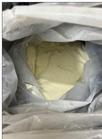
Figure 3. Xanthan gum powder is used as a dry additive in the sand-column infill.
