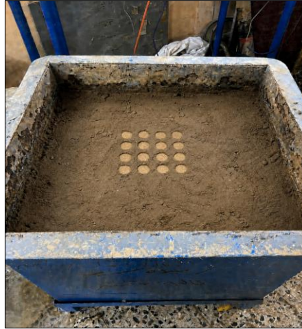
Figure 7. Layout of the 4 \times 4 sand columns embedded in the clay bed prior to placement of the 50 mm sand cushion.
