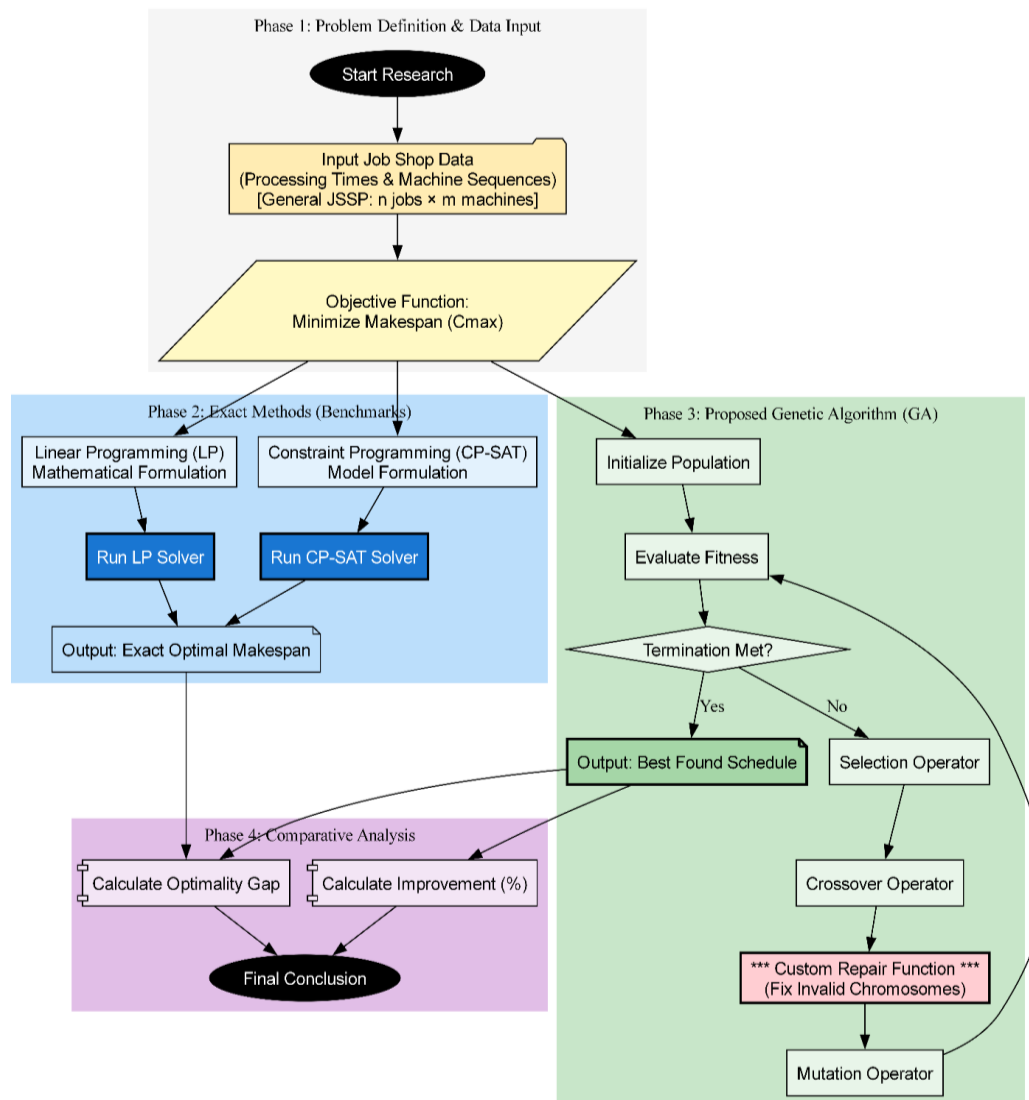
Figure 1. Methodological flowchart of the proposed four-phase comparative optimization approach.
