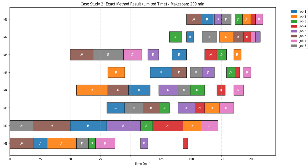
Figure 4. Gantt chart of the optimal schedule for Case Study 2 (8×8) using the exact CP-SAT method.
