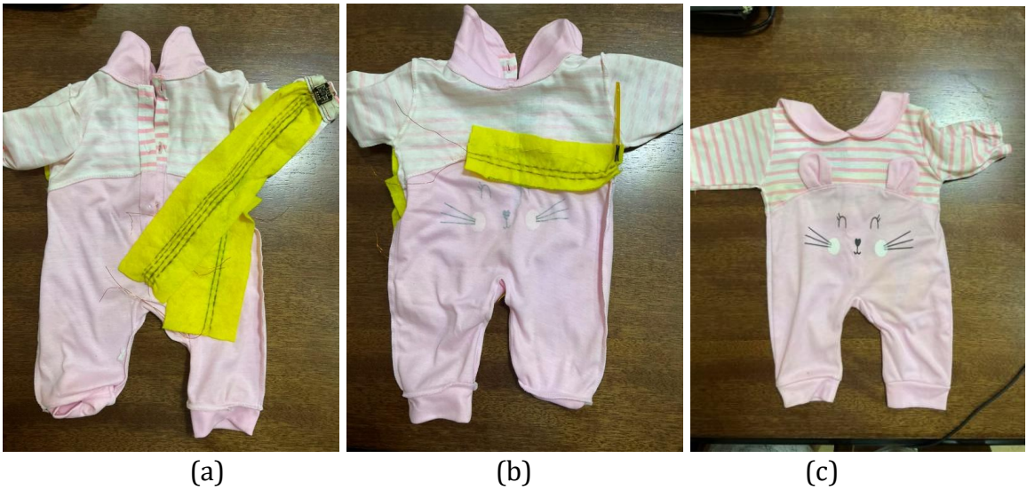
Figure 5. Wearable assembly: (a) sensor wiring on fabric (b) garment integration (c) external prototype view.
