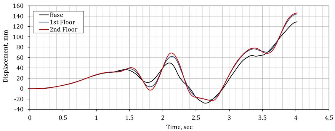
**Figure 8.** Displacement-Time History for Elastic and Inelastic Behaviors of the Prototype Building,  $PGA=0.32g$ .
