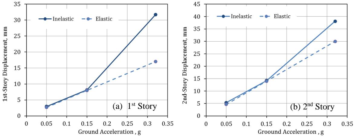
Figure 10. Variation of the Maximum Displacement with Ground Acceleration for both Inelastic and Elastic Behaviors of the Prototype Building (a) 1<sup>st</sup> Story, (b) 2<sup>nd</sup> Story.
