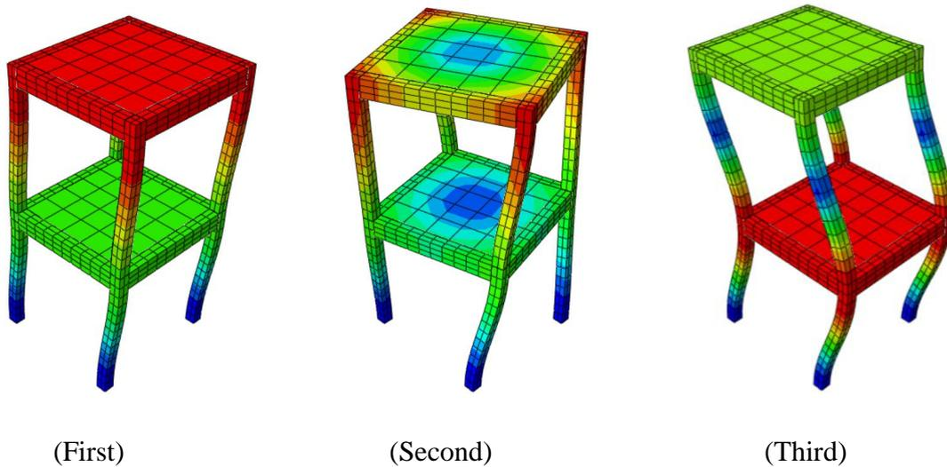
**Figure 5.** Mode Shapes of the Prototype Building.
