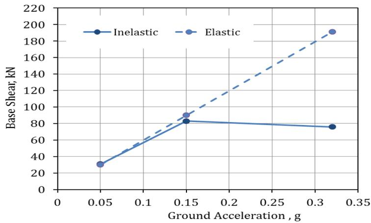
Figure 11. Variation of the Maximum Base Shear with Ground Acceleration for both Inelastic and Elastic Behaviors of the Prototype Building.
