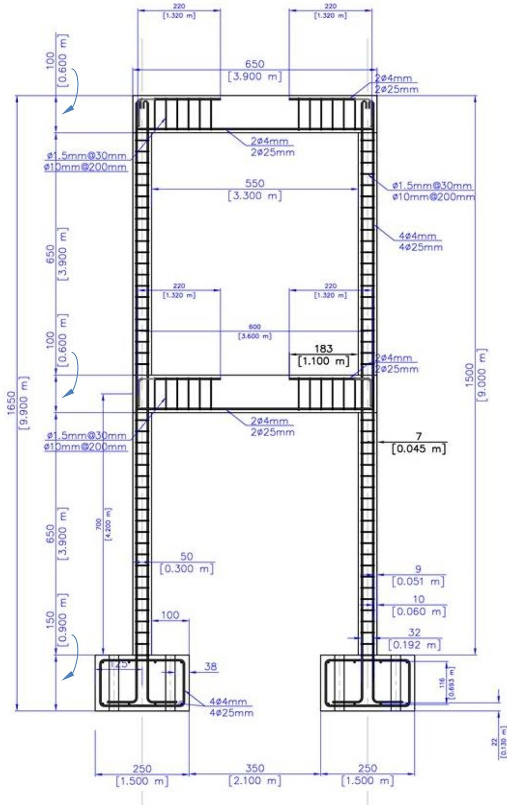
Figure 2. Details of Two-Story 1:6 Scale Model [Prototype] Building.
