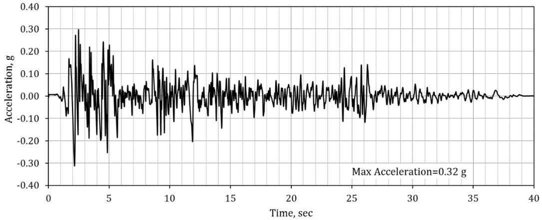
Figure 3. Ground Motion for El Centro 1940 NS Accelerogram Component.
