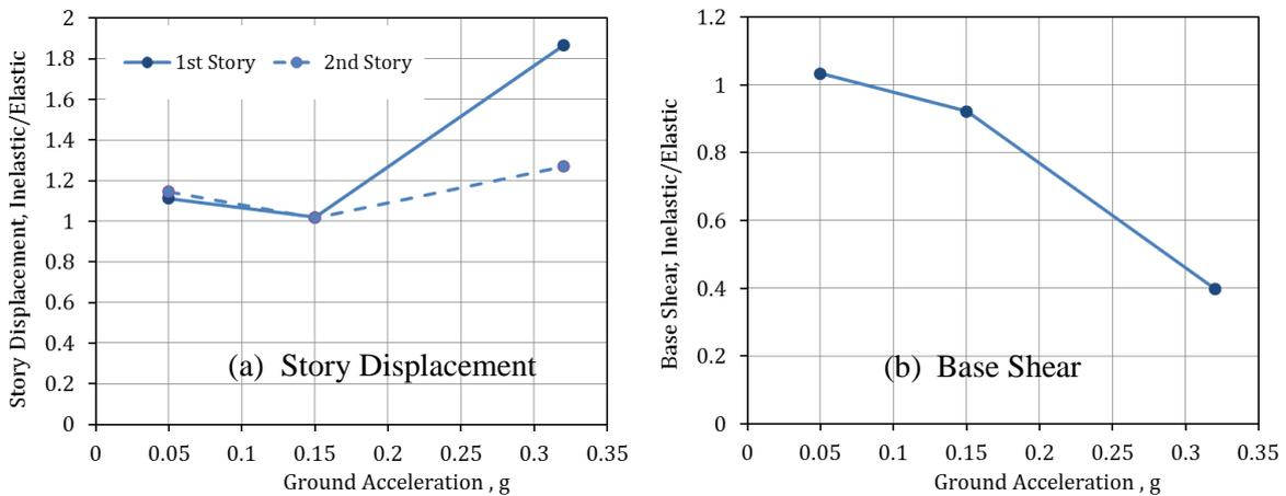
Figure 12. Variation of the Maximum Inelastic/Elastic Response with Ground Acceleration of the Prototype Building, (a) Story Displacement, (b) Base Shear.
