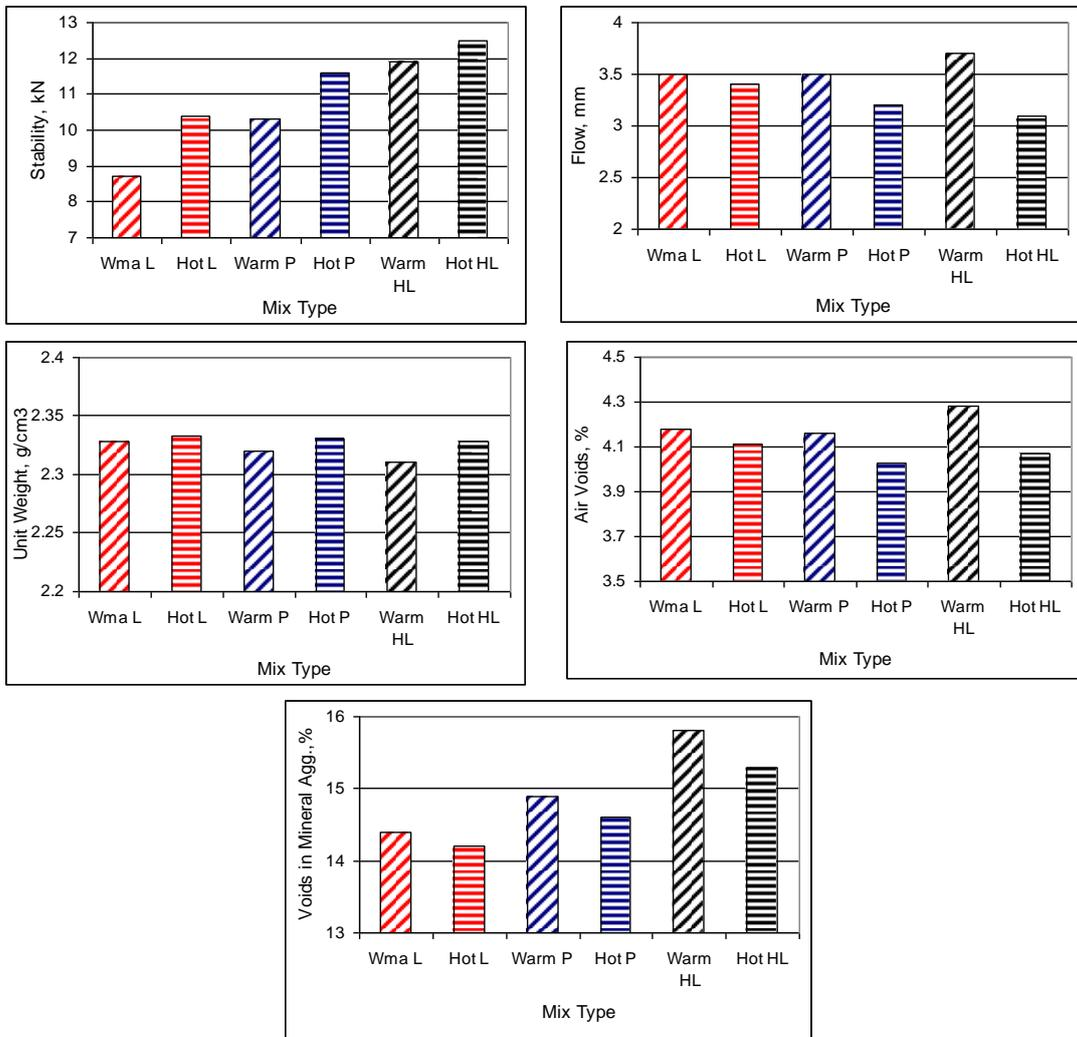
Figure 8. Effect of mix types on Marshall properties.
