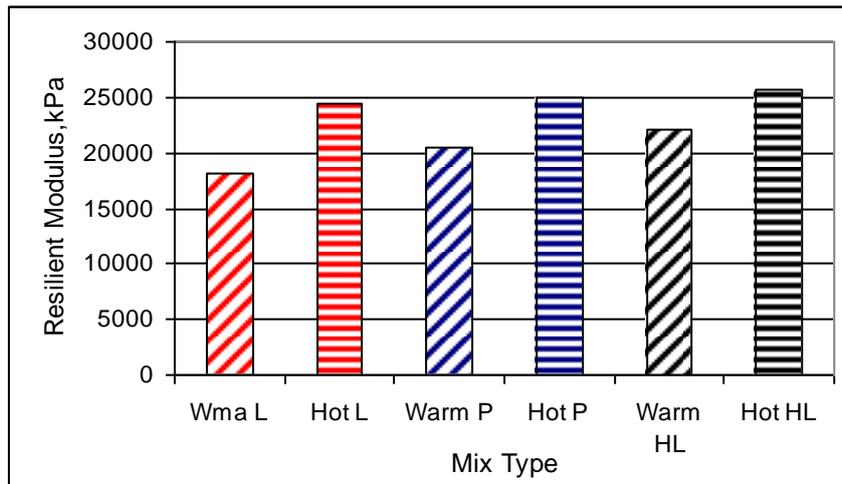
Figure 12. Results of resilient modulus.
