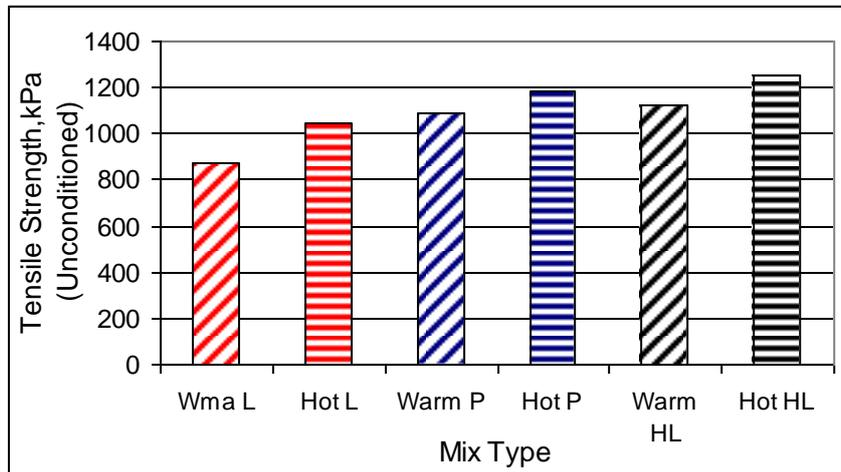
Figure 10. Unconditioned Indirect tension test results specimen.
