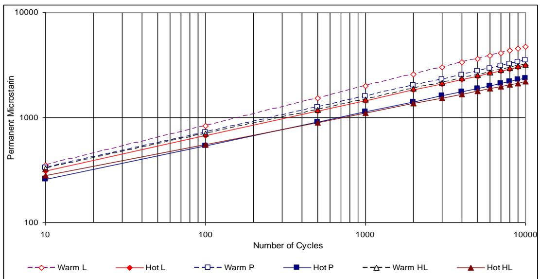
Figure 14. Results of permanent deformation test.
