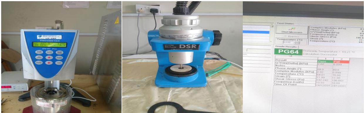
**Figure 1.** Photograph for asphalt cement PG test
