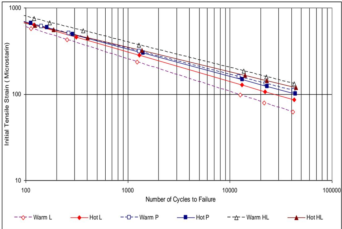
Figure 15. Effect of mix type on fatigue performance.
