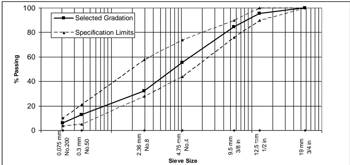
**Figure 2.** Selected aggregate gradation and specification limit
