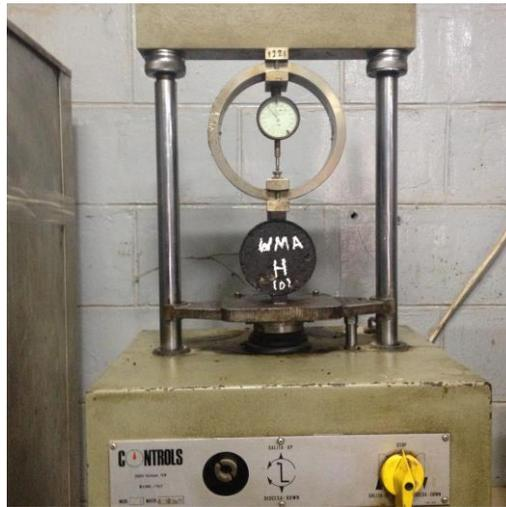
Figure 9. Indirect tension test for WMA specimen.
