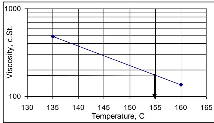
**Figure 5.** Viscosity – Temperature chart of PG 64-16.
