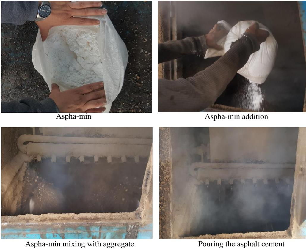
Figure 3. Aspha-min, addition and mixing method.
