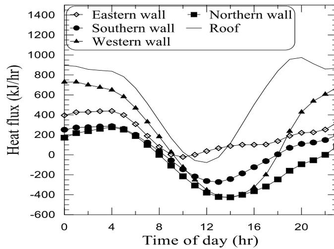
Figure 8. The Variation of the heat flow rate from zone construction to the room with time.
