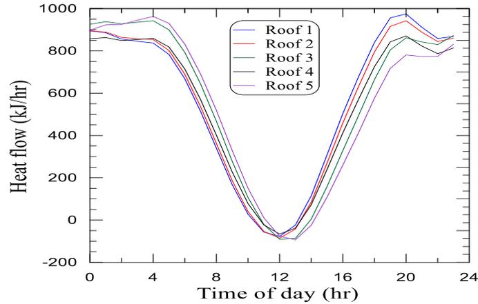
Figure 10. The effect of roof type on the heat flow to the room from the roof.
