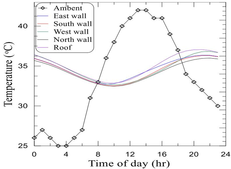
Figure 7. The Variation of inside surface temperature of the zone construction with time.
