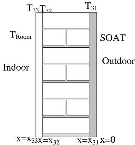
**Figure 1.** The cross section in typical three layered wall.
