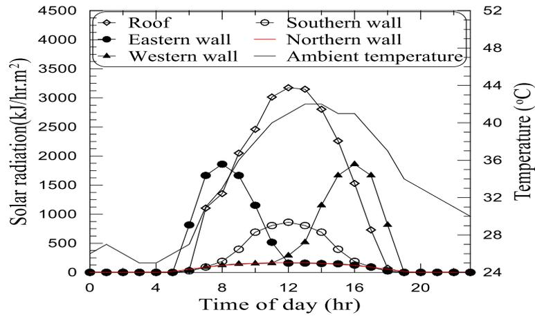
Figure 4. The Solar Radiation Intensity on Different Surfaces and ambient Temperature in Baghdad.
