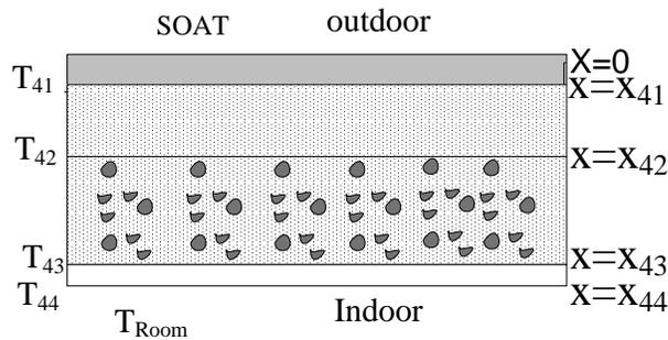
**Figure 2.** The cross section in 4 layered roof.
