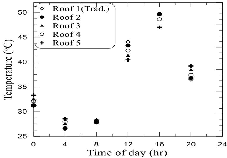
Figure 5. The inside surface measured temperature along the day for the roofs under study.
