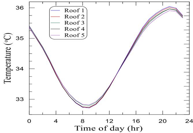
Figure 9. The effect of roof type on the inside room temperature.
