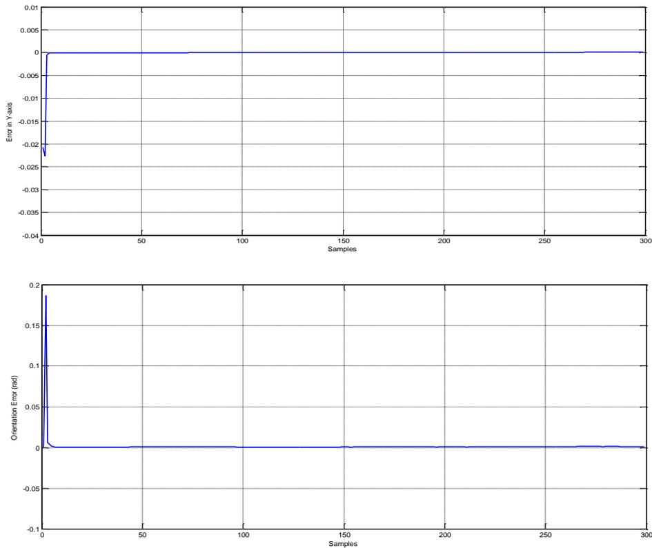
Figure 20. Pose error of the mobile robot: a) error in X-axis; b) error in Y-axis; c) orientation error.
