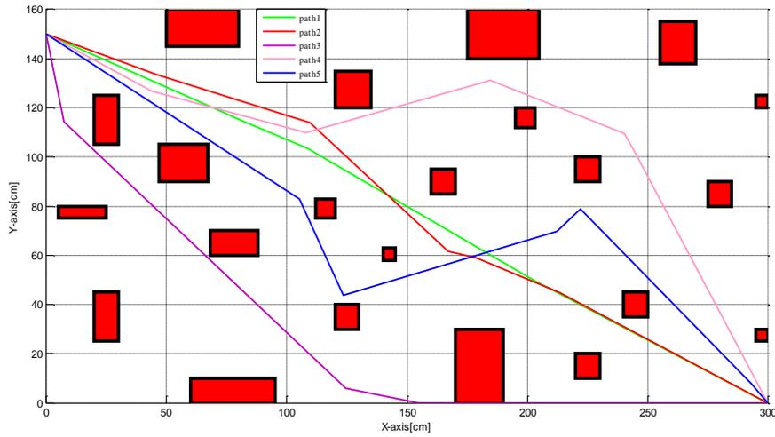
Figure 14. The optimal paths using the ABC algorithm.
