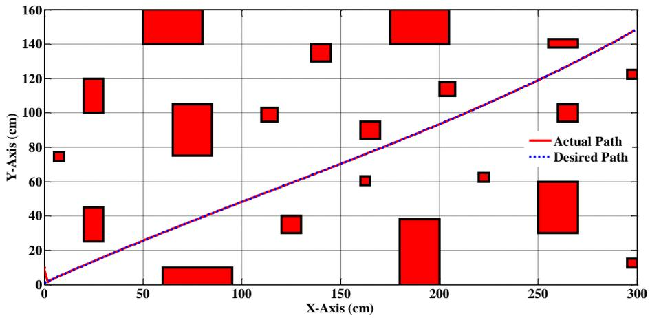
Figure 7. The reference path equation and actual path for a mobile robot.
