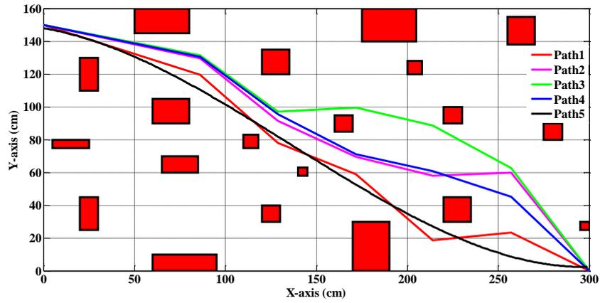
Figure 13. The optimal paths using PSO algorithm.
