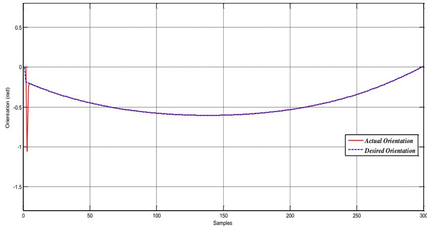
**Figure 16.** The desired and actual orientation for a mobile robot.
