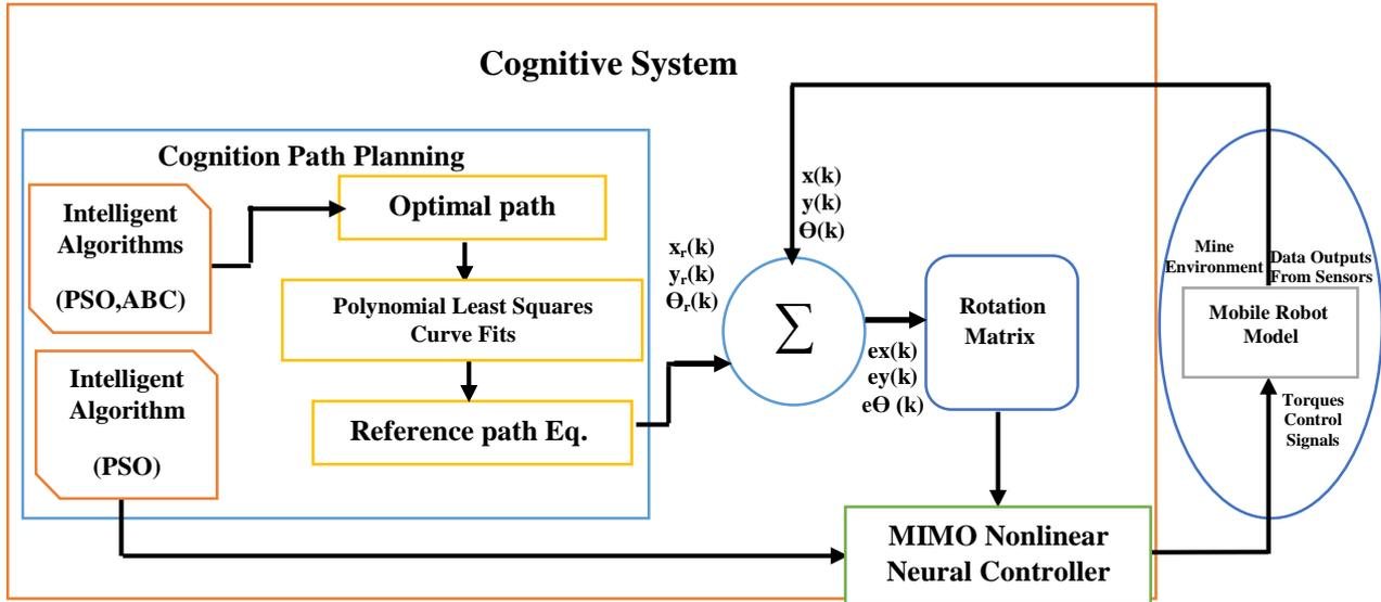
**Figure 2.** The mine mobile robot cognitive system structure.
