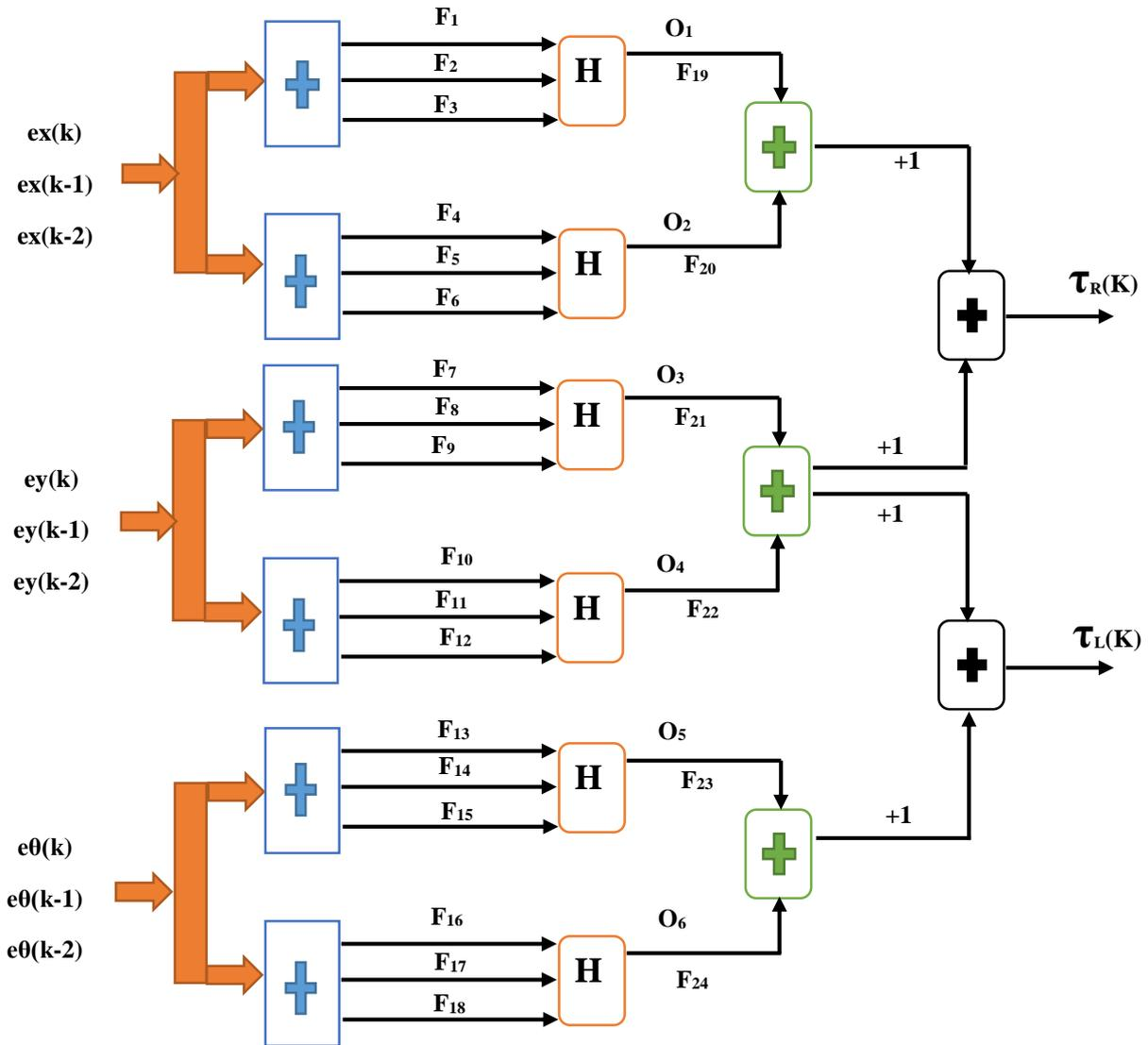
**Figure 3.** The proposed MIMO nonlinear neural controller structure.
