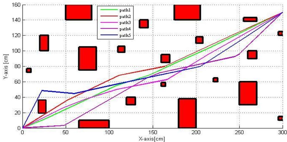
Figure 6. The optimal paths using the ABC algorithm.
