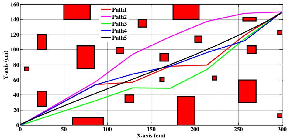
Figure 5. The optimal paths using PSO algorithm.
